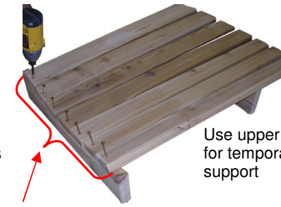
Center Back Slats on Lower Canoe with Pre-drilled screw holes on top
