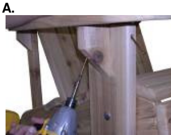
1. Attach arm rests to supports with 3" Screws 2. "Toe Nail" Screws through front and back edge of front leg with 3" screws
