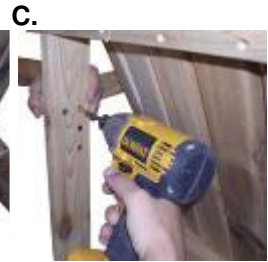
Attach arms to back legs with 1-5/8" screws
